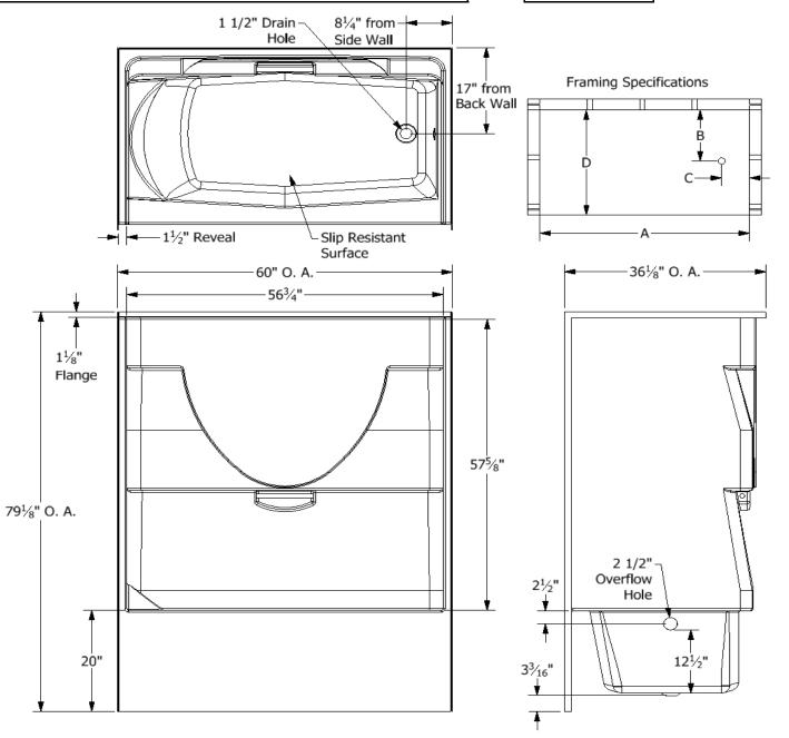
Certified to conform to HUD/UM73b,ANSI Z124.1, and ASTM E- 162 Flame Spread Rating 200 or less and is under a program of factory inspection.
